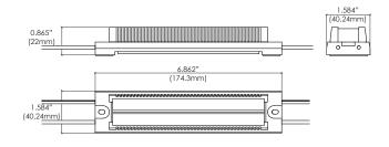
Cyclops Body, I module per foot 850 lm/ft(OTSC-LI-BW65), 12 linear ft max load on ASU-100-24U
